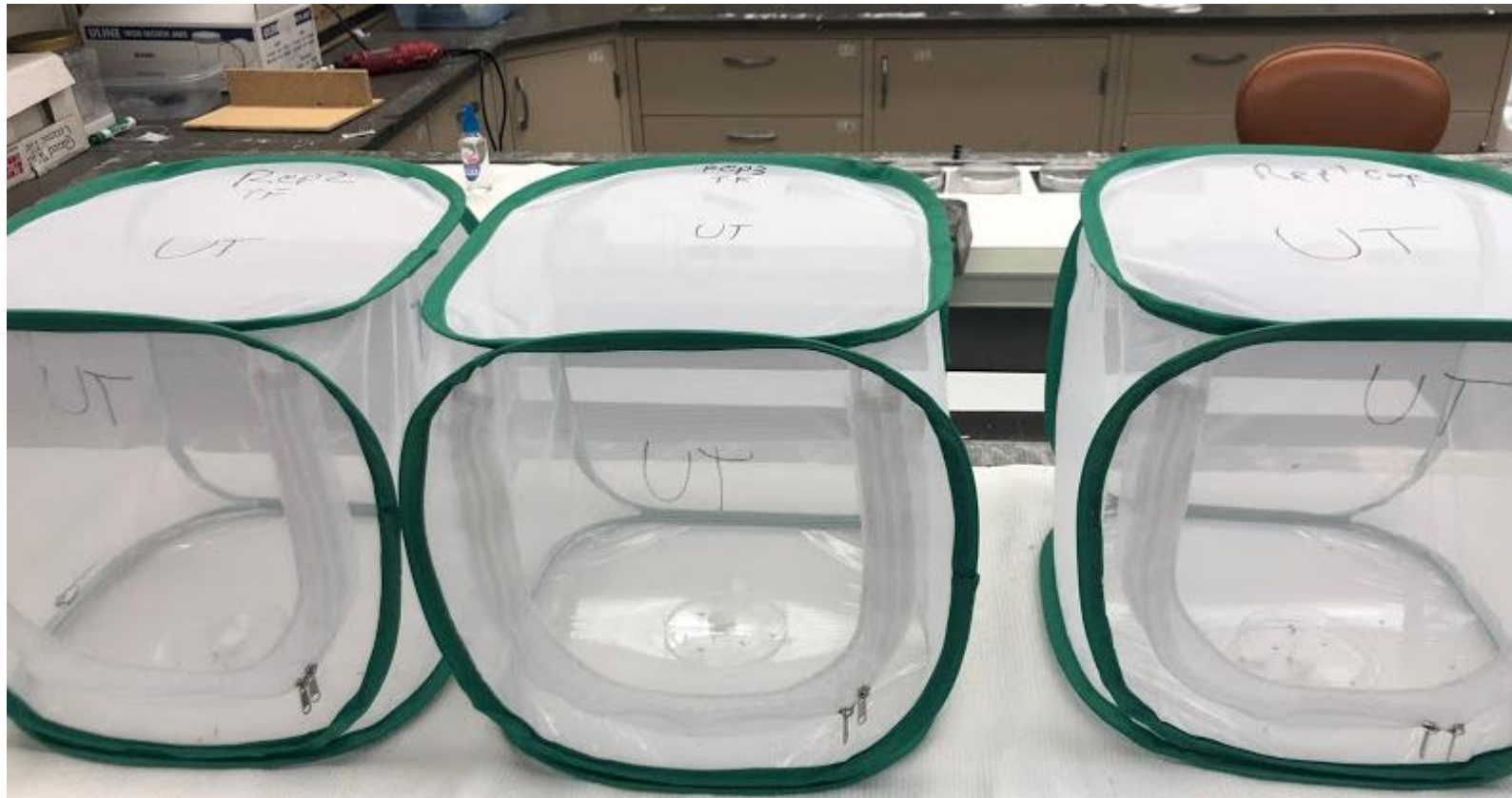
Figure 6. Photos of cages used for the fresh (wet) residue repellency test of the Mosquito Free/ Tick Free product. Each side of the cubical cage was 12 x 12 inches in size.
